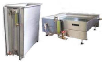
According to the standard, each sample should be subjected to 10 heating and cooling cycles. The sample should be heated in an oven and cooled in accordance with the two different methods,
